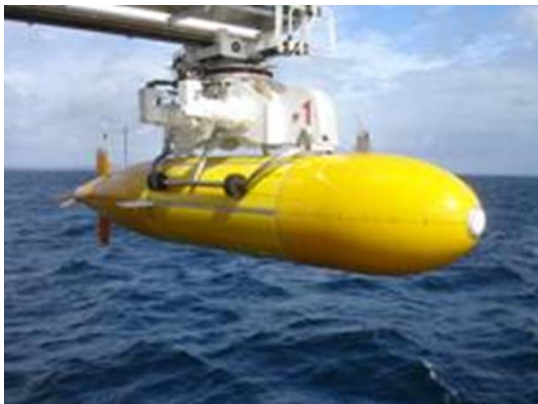
Fig. 1. Autosub 6000 of the National Oceanography Centre at the University of Southampton that can reach an ocean depth of 6km.
